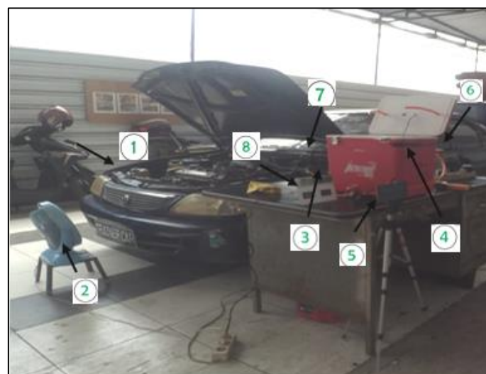
Figure 2. Photographic view of apparatus: (1) Engine; (2) Extra fan; (3) Themocouple; (4) Cooling box; (5) Recorder; (6) Battery; (7) LPG Evaporator; and (8) Temperature displayer.
