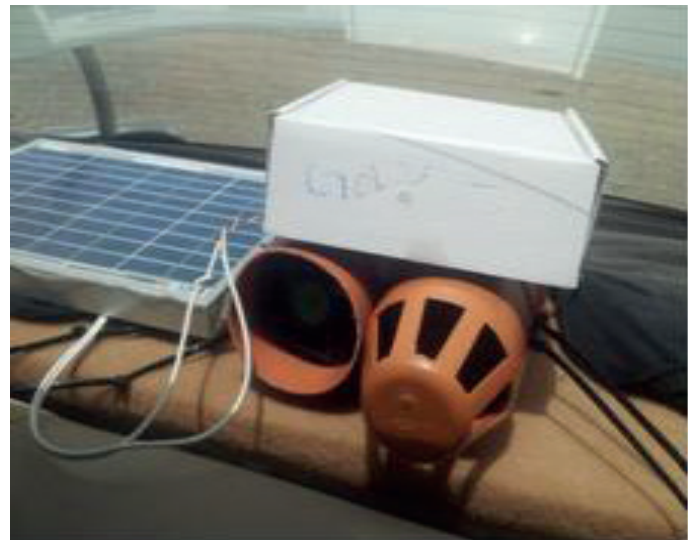
Fig. 8 Ventilation system mounted on the rear end of the car (Vishweshwara et al., 2013).
