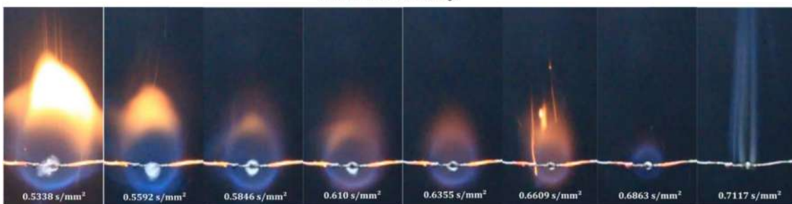
Fig. 5. Single droplet combustion of 25% v/v fraction mixture.
