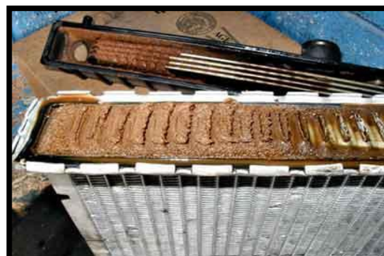
Gambar 1.2 Upper Glower Tank Radiator
