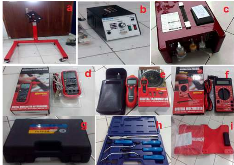
Gambar 11. Peralatan Bantu, Pengukuran dan Diagnosis IBIKK: (a) Engine Stand, (b) CDI and Sparkplug Checker, (c) Engine Gas Analyser, (d) Multitester Tipe 1, (e) Tachometer Noncontact, (f) Multimeter Tipe 2, (g) Radiator Cup Tester (h) Brake Tools dan (i) Creeper.
