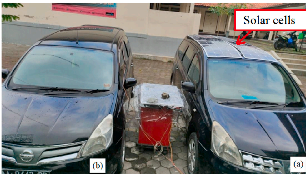
Fig. 1. The test vehicle placement: (a) with a car cabin cooler and (b) without a car cabin cooler.
