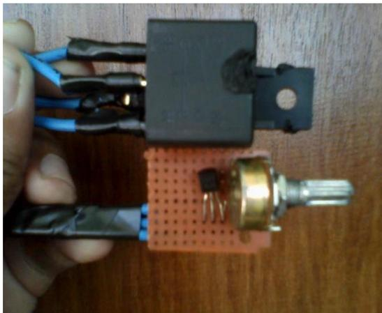
Gambar 4.2. Rangkaian *fuel cut off*
